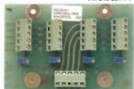
Load Cell Trim Board, Parallel four load cell
