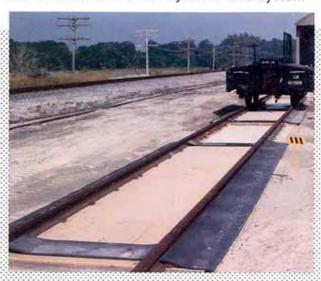
is sold as a configuration of modules measuring 12'6" and 25'0" long. With the proper configuration, virtually any length of rail car (from the shortest to the longest) can be weighed.
