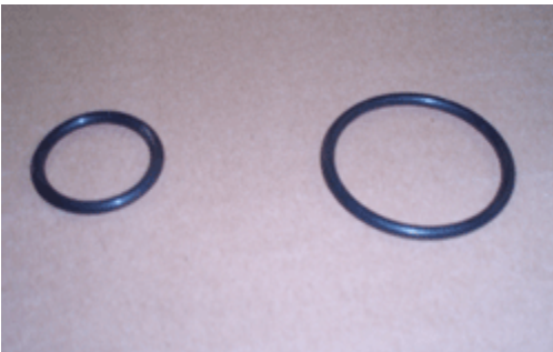
“O” Rings two sizes each receiver cup uses one of each P/n 412-3041-0 1/8” x 1 1/8” x 1 3/8” P/n 412-3040-0 1/8” x 1 7/8” x 2 1/8”
