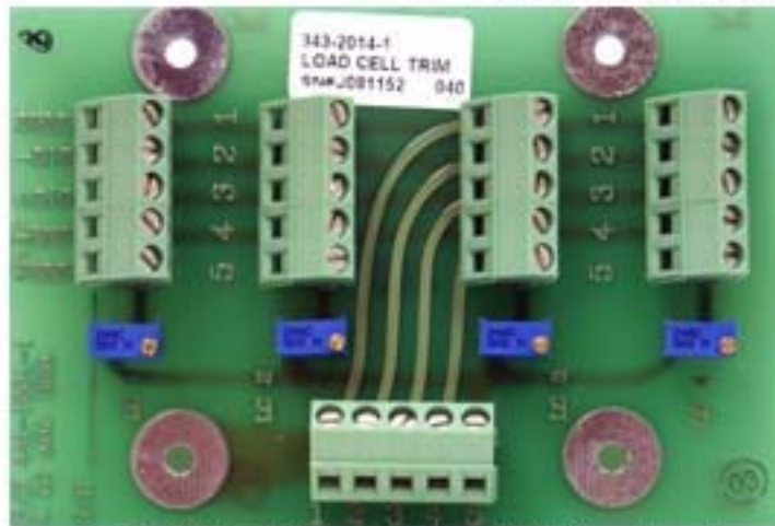
Load Cell Trim Board, Parellel four load cell
